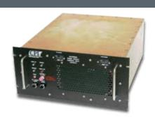
to shape the voltage pulse to ensure low-jitter operation and the magnetron filament DC filter are all contained in this oil tank. The magnetron is mounted external to the high voltage tank for ease of replacement. External fans are provided to cool the magnetron. Both it and the solid-state switch are thermally interlocked as they can be damaged if sufficient cooling is not supplied.
